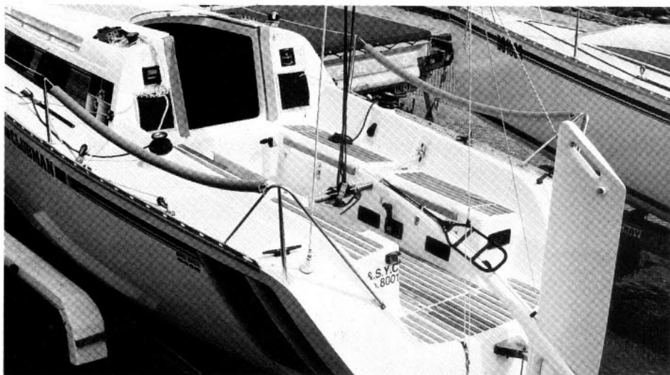
LEFT: Cockpit has teak slats on floor and seats and inset teak foot rests. Controls for the outboard and vents for its compartment are under the traveller. RIGHT: Halyards and sail control lines are tunneled under the cabin top.
