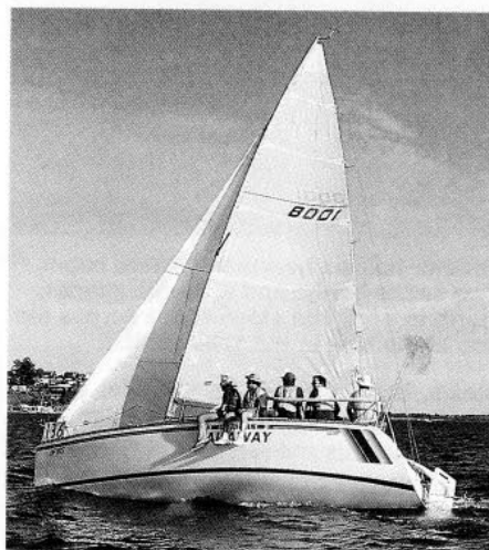
Sail plan is high aspect with not much roach in the mainsail.
